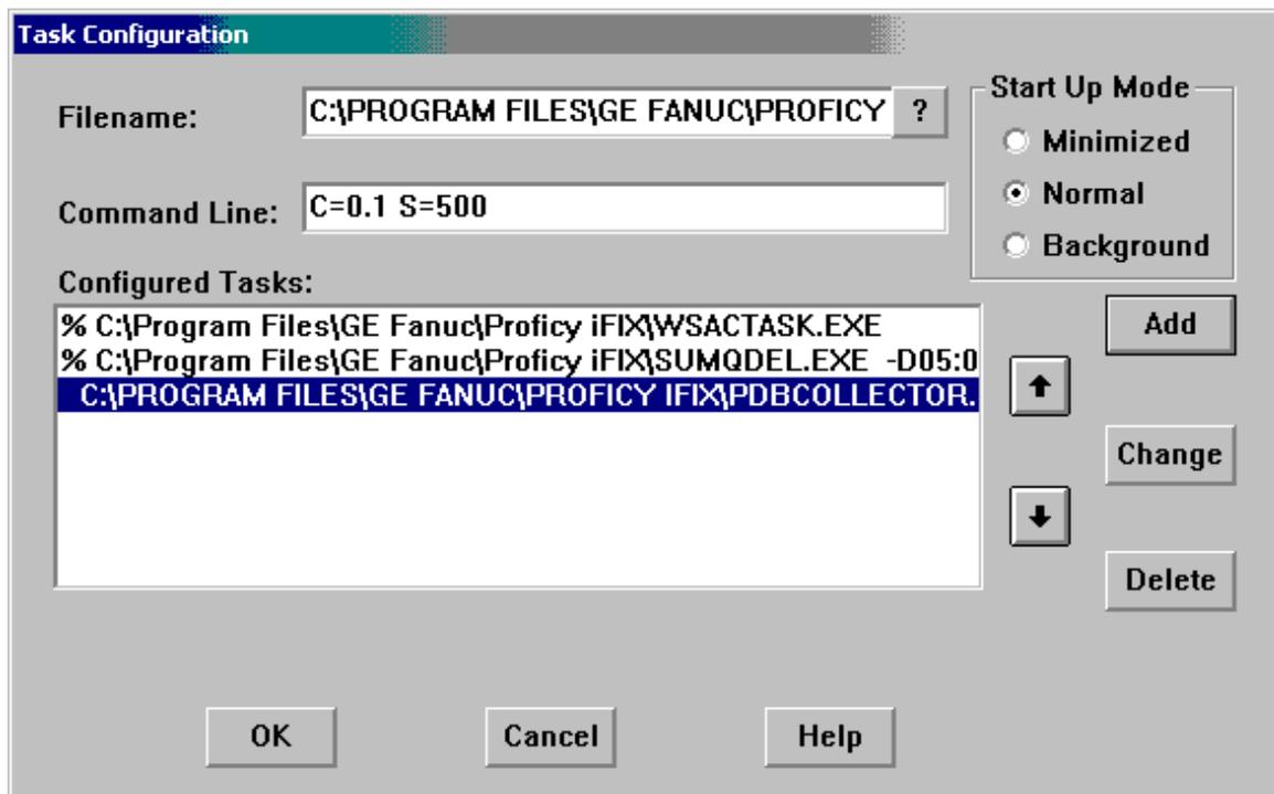
Figure 1: Automatic startup of EDA collector
