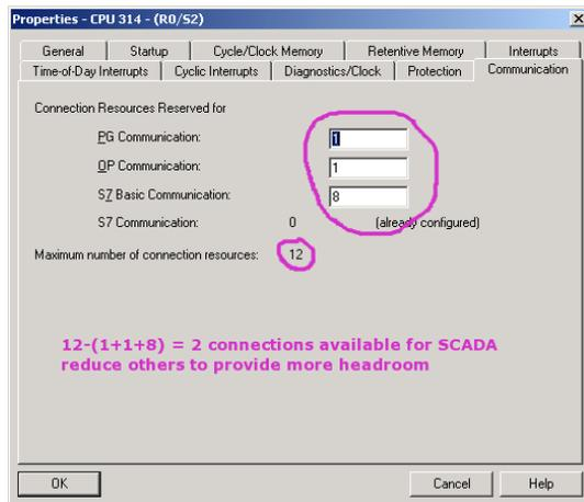
\*\*Note - by default the driver uses SCADA connections, which are the missing/unlisted connections in the picture above. The S7 Basic connections are PLC-PLC connections normally you can reduce this number. Ideally you want the SCADA connections free to be at least 2+the number of SCADA's. To force the driver to use an OP or PG connection set the local TSAP to "R=0;S=2;OP" or "R=0;S=2;PG"
